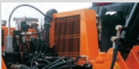
Oil cooler with thermostat
